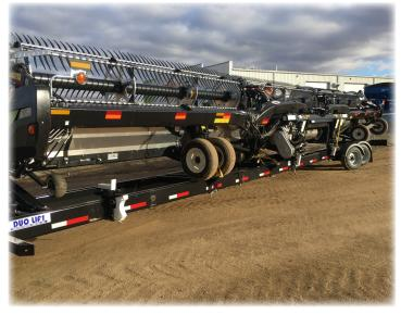
Adjustable and adaptable header supports for mounting all types and sizes of headers with ease. Shown above, with 50' Flex Draper head.
