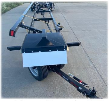
801003 - The All Steer Head Hauler features extended coverage front steel fenders with gravel guard.
